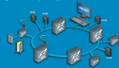
The FTA consists of a Master Controller (MC) and Door Interface Modules (DIM). The MC and DIMs are designed with an Open Standards Operating System utilizing Hydra Protocol to provide the highest level of system operations and reliability. The DIM is currently offered in a Dual Door Module (DDM) or Single Door Module (SDM).
